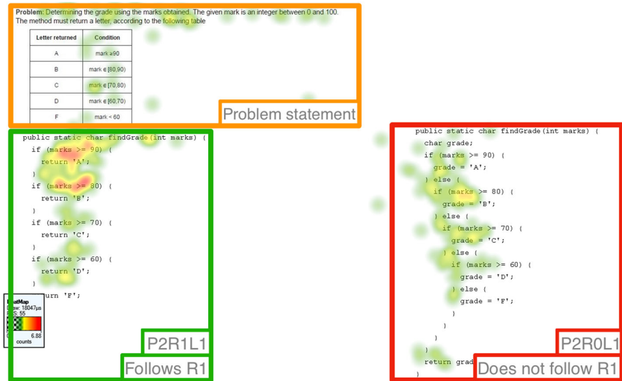
Fig. 2 A screenshot from one participant for R1: minimize nesting with the left ( P_2R_1L_1 ) following the rule and the right ( P_2R_0L_1 ) not following the rule. The method functionality is given on top. A gaze heatmap is overlaid on top, which illustrates where a participant directs their attention on a screen, with warmer colors denoting a higher concentration of gazes
